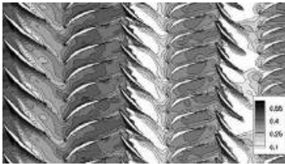
Fig. 6. Instantaneous axial velocity flow field, partial mass flow operating point (large gap configuration, h/H=94\% )
