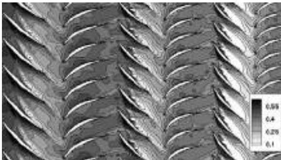
Fig. 5. Instantaneous axial velocity flow field, partial mass flow operating point (small tip gap configuration, h/H=94\% )
