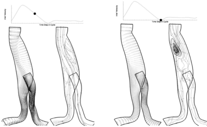
Fig. 4a. Velocity and instantaneous streamlines along the lateral surface at two different times for the stented AAA patient
