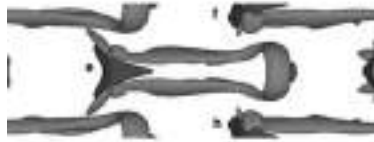
Fig. 7. Illustration for counter-rotating-vortices shocks (top view)
