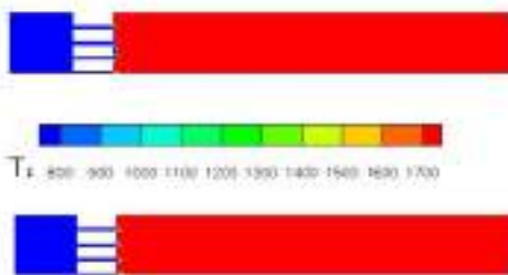
Fig. 19. Contours of temperature; Top: flame held at solids. Bottom: flame held at flame holder in clean channel
