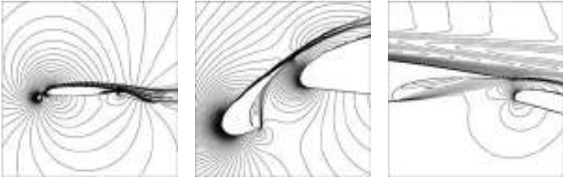
Fig. 2. Mach contours on the final level adapted grid: Full view (Left), close to slat (Center) and close to flap (Right) ( \alpha = 20^\circ ). Contour levels are 0:0.01:1.03
