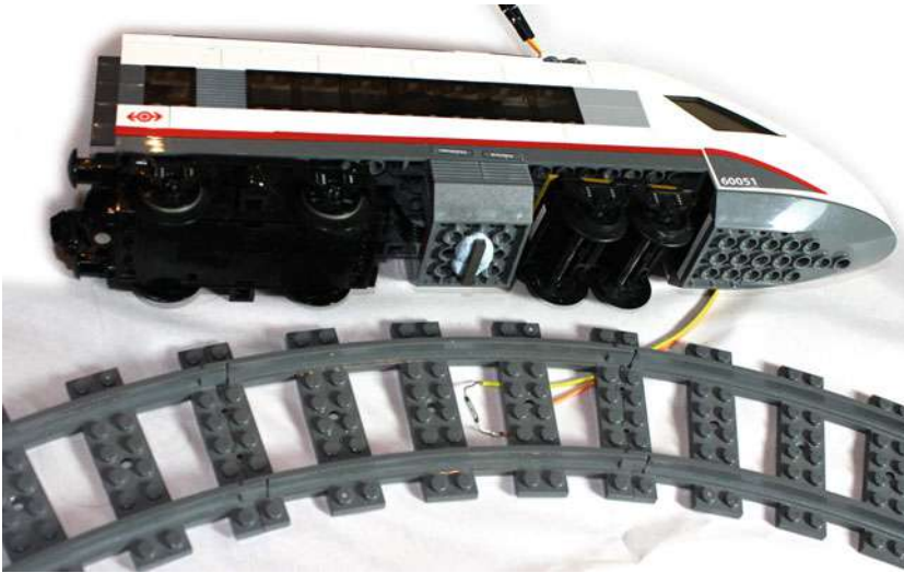
Figure 6-5. Reed switch mounted under the Lego train track and magnet on the train
