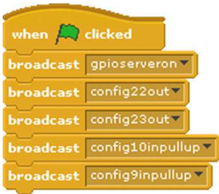
Figure 3-14. Setup code for Robot Soccer game added to the Stage Scripts tab
