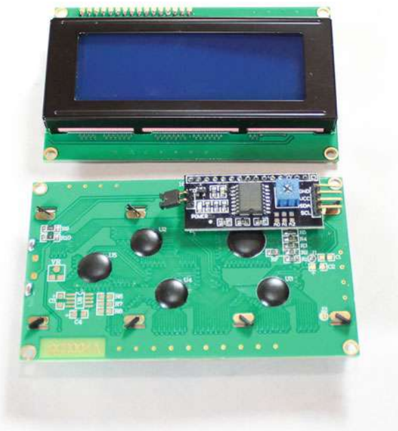
Figure 5-13. Photo of the LCD character display and backpack mounted on the rear
