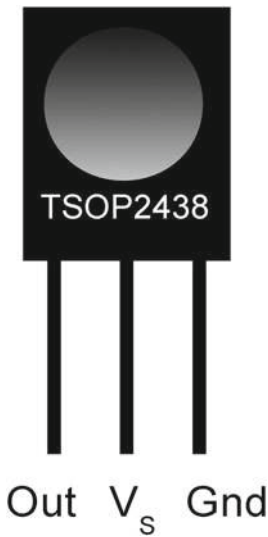
Figure 5-5. Pinout for the TSOP2438 and similar infrared receivers
