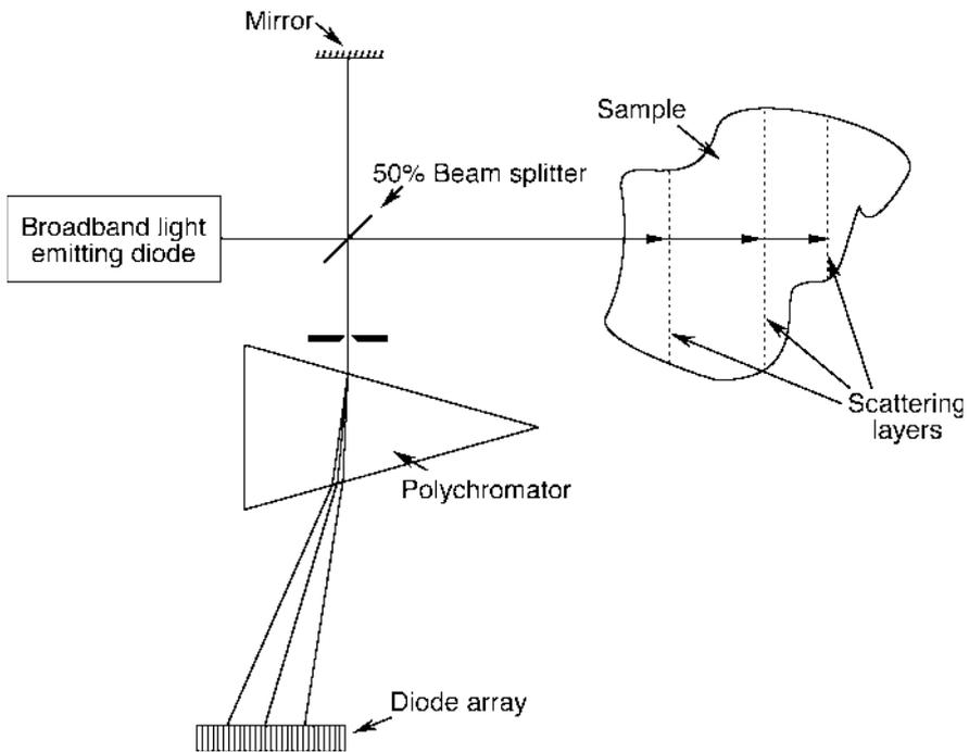
**Fig. 5.11** Spectral domain optical coherence tomography (SDOCT) (Andretzky et al., 1998; Häusler and Lindner, 1998). Polychromatic backscattered light from different depths interferes with polychromatic light of a reference beam. The interference of the beams is analyzed with a polychromator and a multichannel detector. From the spectral changes due to interference, information about the depth of the scattering layer is obtained
