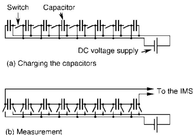
**Fig. 10.22** Generating the high voltage for an IMS (Goebel and Breit, 2000). (a) A set of  $n$  capacitors is charged with the voltage  $V$ . (b) The capacitors are connected together in series for generating the high voltage  $n \cdot V$
