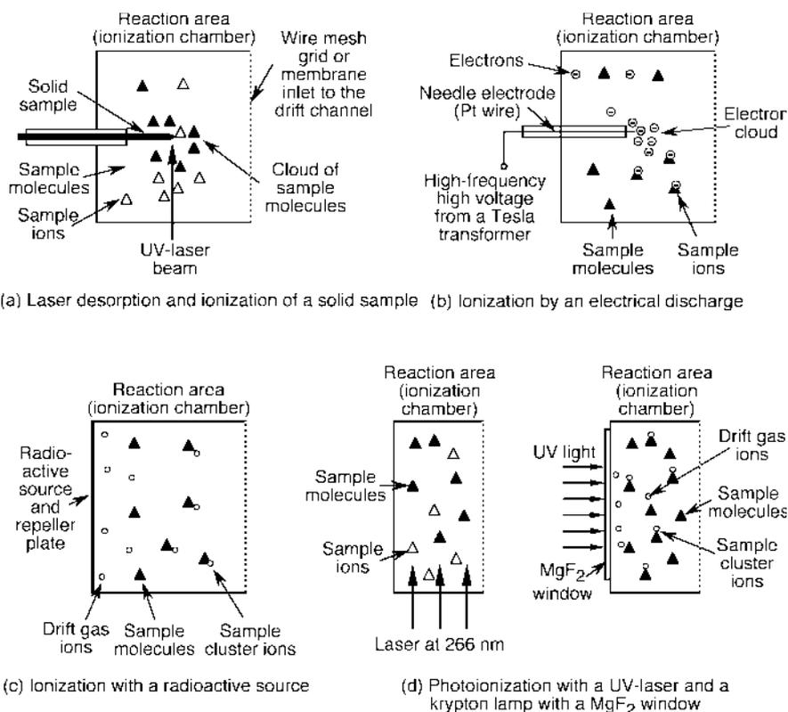
**Fig. 10.15** Examples of ionization methods (see also Table 10.1)
