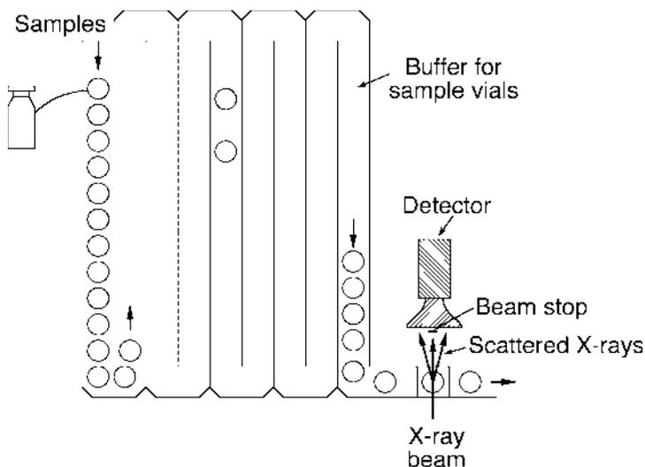
**Fig. 4.37** Automatic SAXS and wide angle X-ray scattering analysis of biological samples. A large number of vials is automatically sampled and production faults immediately are detected and responded to
