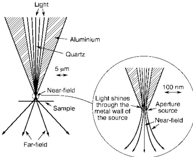
**Fig. 7.31** Optical far-field and near-field in the vicinity of a small optical tip for a SNOM. Since the light can transmit through thin layers of metal, the diameter of the light beam in this design cannot be less than a few 10 nm
