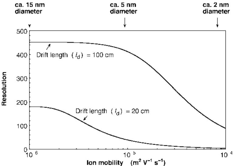
**Fig. 10.9** Theoretical resolution of an IMS at different drift lengths and ion mobilities: long shutter pulses enhance the sensitivity, but limit the resolution for small ions. The parameters in this example are: temperature, 130 °C; drift voltage, 80 kV; initial ion pulse width, 1 ms; shutter pulse voltage, 1000 V; length of the reaction area, 3 mm; distance between aperture grid and Faraday plate, 1 mm; voltage at the aperture grid, 500 V
