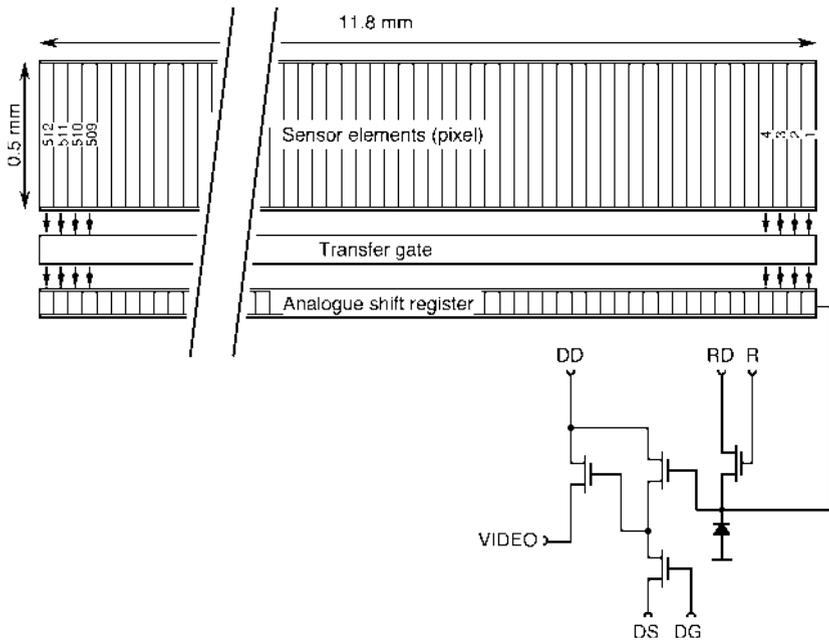
**Fig. 4.21** Linear charge coupled device (CCD). The sensor elements generate electrons by absorption of photons and store the electrons in potential wells. After a certain period of time, the collected electrons are transferred to the analogue shift register and read out. The symbols are: DD, drain of the output amplifier; DS, source of the output amplifier; DG, gate of the output amplifier; RD, drain of the reset transistor; R, clock gate of the reset transistor (Nölting, 1991)
