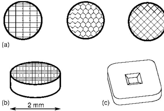
**Fig. 6.7** TEM grids. (a), (b) Some common patterns of TEM grids made from a variety of materials, e.g., platinum, silver, tungsten, molybdenum, stainless steel, or titanium. Among these materials, platinum is the chemically most inert, but expensive. (c) Silicon nitride “grid” with a single window (from SPI Supplies, West Chester, PA)
