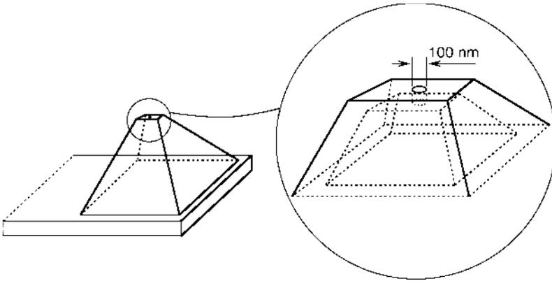
**Fig. 7.30** SNOM tip made from silicon nitride. It was manufactured by using photolithography, potassium hydroxide etching, and electron beam nanolithography (Zhou et al., 1998, 1999)
