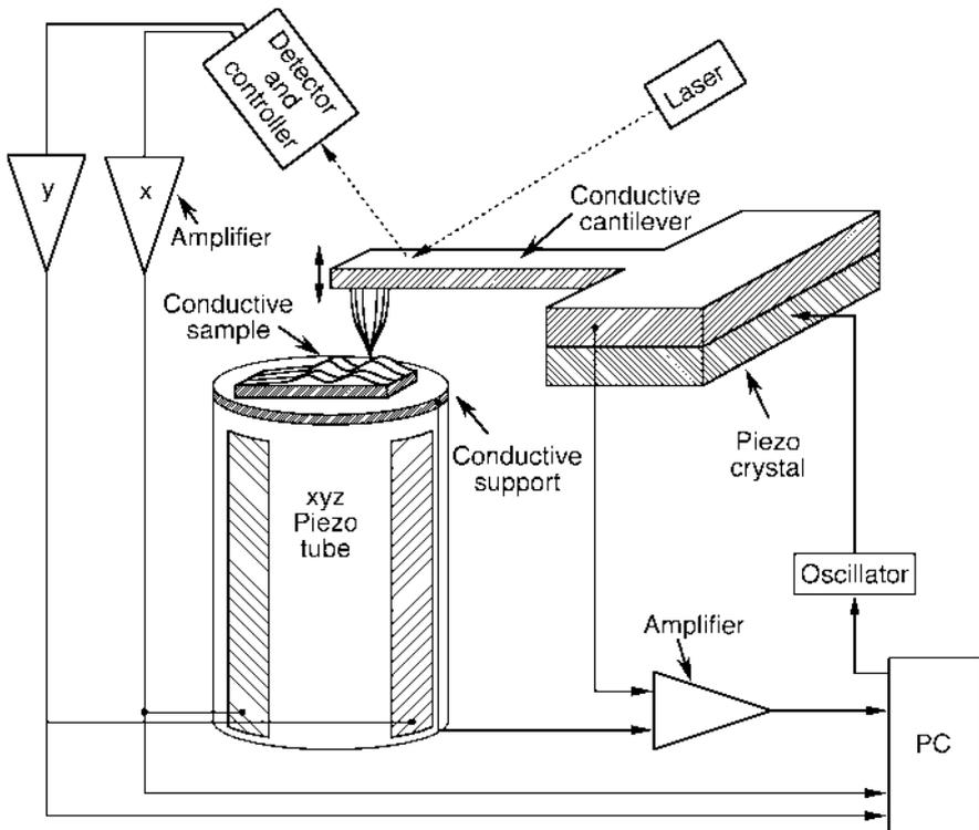
**Fig. 7.37** STM with simultaneous AFM capability: AFM and STM sense different physical properties. The combined information provides greater insight into the chemical nature of the sample and its physico-chemical properties
