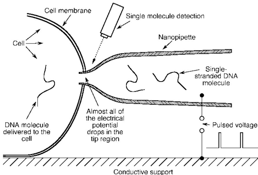
**Fig. 8.22** Programmable delivery of DNA through a nanopipette (Ying et al., 2002; Bruckbauer et al., 2002b). The conical geometry of the pipette causes most of the electrical potential drop to occur in the tip region. Pulsatile delivery of DNA molecules is achieved by controlling the applied voltage
