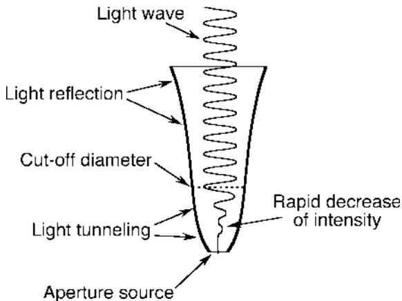
**Fig. 7.29** Propagation of a light wave in a SNOM probe tip. Up to the cut-off diameter (about equal to the wavelength), the light travels with only little attenuation. Beyond this critical diameter, the light intensity very rapidly falls off
