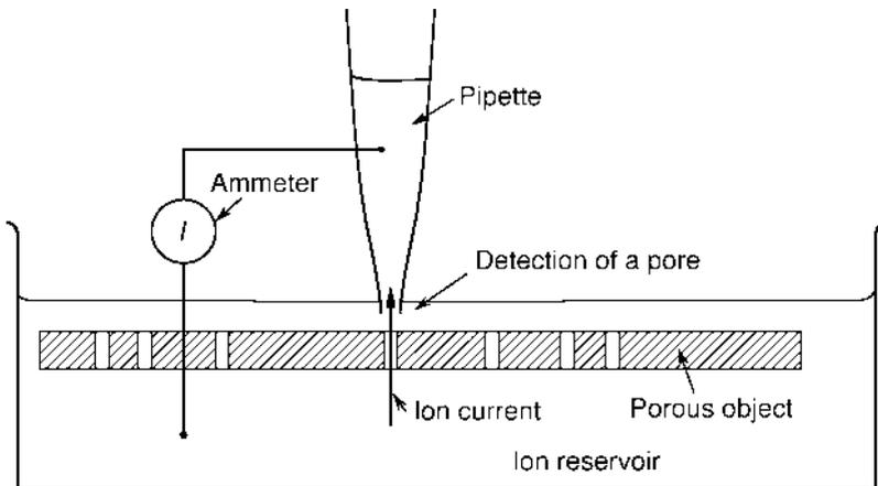
**Fig. 7.35** Detection of membrane pores by a scanning ion conductance microscope. The probe is a nanopipette filled with electrolyte solution. The current between pipette and ion reservoir starts increasing when the pipette tip approaches a pore. The technique permits 100-nm resolution characterization of distribution and sizes of pores
