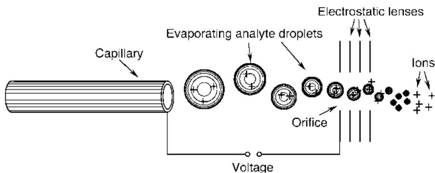
**Fig. 3.11** Electrospray ionization method. Analyte solutions delivered by liquid chromatography or a syringe pump are sprayed through the narrow, heated capillary leading into the mass spectrometer. A voltage of typically 200 V – 5 kV is applied between capillary and orifice in front of the electrostatic lenses. Ions form in vacuum by evaporation of the analyte solution of charged droplets
