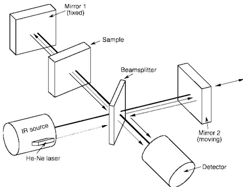
**Fig. 5.3** Typical design of FTIR spectrometers. The lamp, e.g., a thermal source, emits a beam of infrared radiation. A Michelson interferometer, consisting of a beamsplitter, a fixed mirror and a moving mirror, splits the beam into two beams and generates an interference of them. The sample inserted in one of the beam paths changes the interference. Interferograms with and without sample are recorded and the absorption of the sample is calculated by inverse Fourier transform (see Fig. 5.6)
