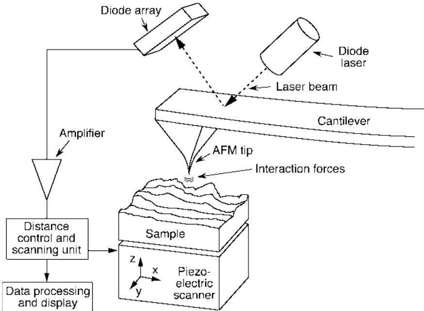
**Fig. 7.1** Principle of operation of an atomic force microscope. A very sharp tip attached to a tiny cantilever probes the sample surface. An optical system comprised of diode laser and detector, e.g., a diode array or a position-sensitive diode, senses the bending of the cantilever and thereby the distance-dependent tip-sample interaction force. For scanning the surface, the sample is moved by the piezoelectric scanner (Binnig et al., 1986)
