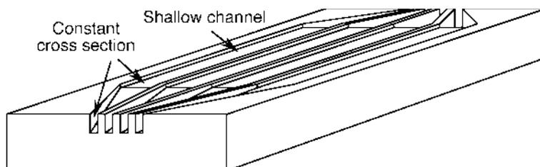
**Fig. 9.9** Simplified example for lab-on-a-chip technology (see, e.g., Swedberg et al., 1996; Swedberg and Brennen, 2001; Cheng et al., 2002; Figeys 2002b, Laurell and Marko-Varga, 2002). Tiny channels are microfabricated or etched into the support. The top is then sealed with another plate (not shown). A single chip may contain all the channels, switches and reservoirs necessary for complicated multi-stage chemical reactions
