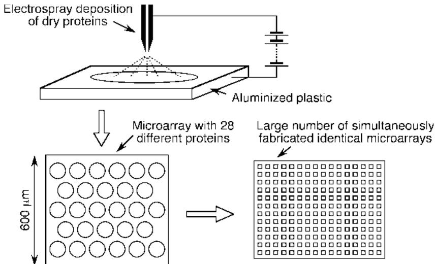
**Fig. 8.24** Electro spray deposition of dry proteins for the fabrication of microarrays and nanoarrays (Avseenko et al., 2001, 2002). These arrays can detect antibodies in plasma samples from mice immunized with the proteins used for the arrays
