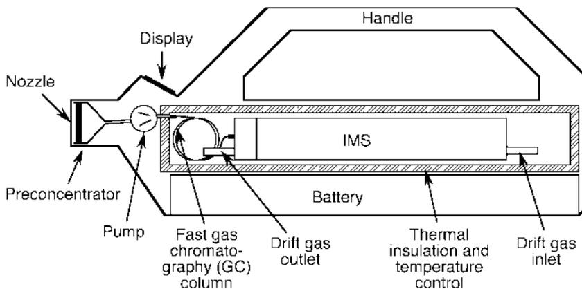
**Fig. 10.12** Hand-carried sniffing detector which further comprises a fast gas chromatography (see, e.g., Snyder et al., 1993). The combination with GC improves the false alarm rate for the detection of dangerous substances by typically one order of magnitude
