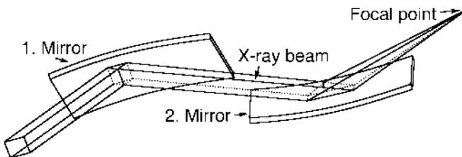
**Fig. 4.30** A pair of X-ray mirrors with grazing incidence focuses an X-ray beam to a spot
