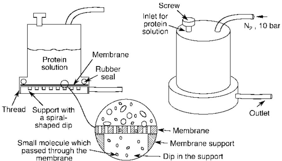
**Fig. 2.16** Ultrafiltration device (supplied, e.g., by Amicon Inc., Beverly, MA). Pressurized nitrogen from a nitrogen flask presses the protein solution against the membrane. Small molecules pass the membrane and are collectable at the outlet. Large molecules stay in the ultrafiltration vessel
