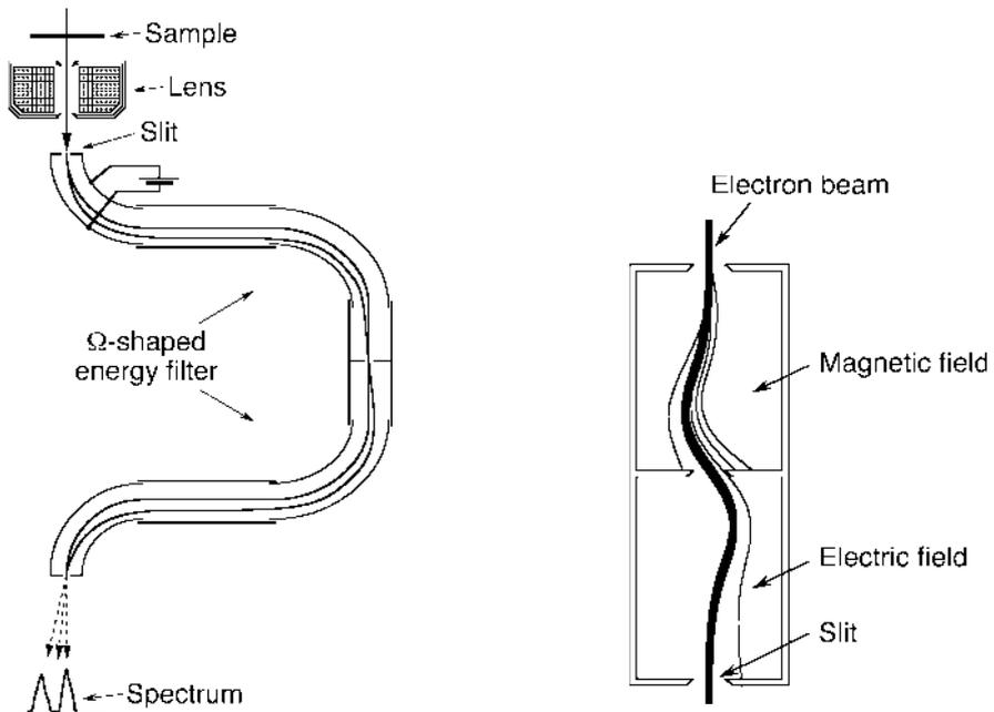
**Fig. 6.15** Two types of dispersive elements for energy filtering of the electron beam to eliminate inelastically scattered electrons, removing the diffuse background and thereby enhancing contrast, or to perform a chemical analysis of the sample. *Left:*  $\Omega$ -filter. *Right:* filter using magnetic and electric fields
