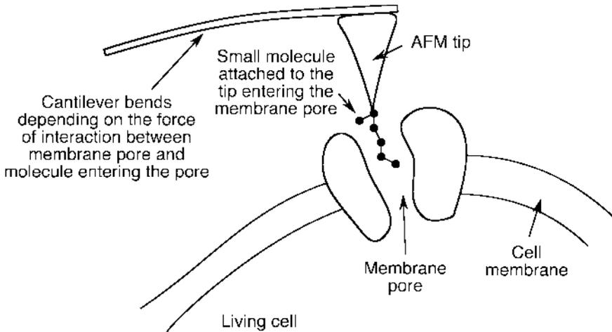
**Fig. 8.11** Nanobiosensor using the cantilever of an AFM (Pereira, 2001). Entering or exiting of specific molecules, including medications, from living cells is observed in real-time and the force of interaction measured
