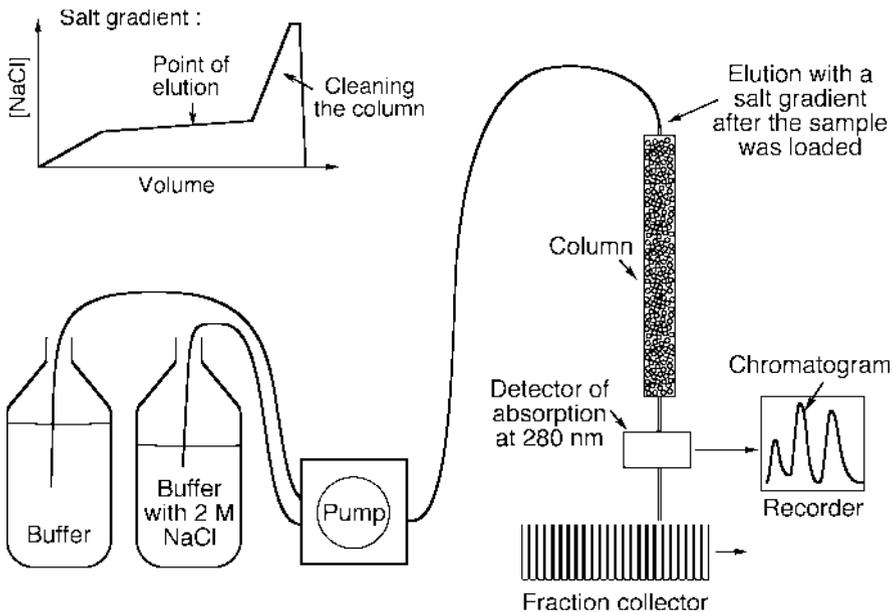
**Fig. 2.6** Typical setup for chromatographic purification of proteins with ion exchange FPLC. The pump mixes the salt gradient for sample elution after the sample was loaded, e.g., with a syringe
