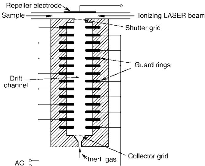
**Fig. 10.19** IMS with an oscillating electric field of the guard rings instead of a constant electrostatic field. Only ions of which the movement is in phase with the oscillating electric field can pass through the drift channel and reach the collector. For further details on frequency-domain IMS see, e.g., Martin et al., 1998
