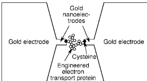
**Fig. 8.21** Conduction between nanoelectrodes through a single molecule (Reimers et al., 2002) or a few organic molecules forming a nanocrystal (Rinaldi et al., 2002). In some cases, rectifying behavior is observed, e.g., for deoxyguanosine nanocrystals (Rinaldi et al., 2002)
