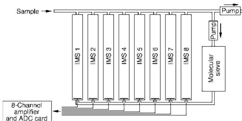
**Fig. 10.26** A multichannel ion mobility spectrometer. For an 8 times higher sampling rate than a single-channel spectrometer, all channels are operated in the same way. For decreased rate of false identifications, one sample may be distributed over different channels that are operated in different modes (see, e.g., Turner, 1993)
