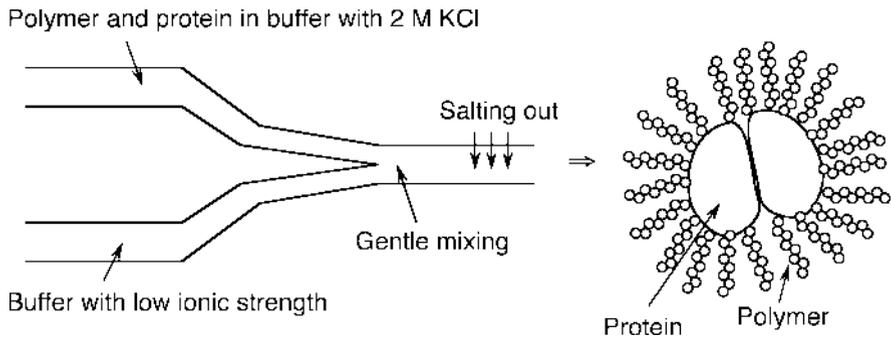
**Fig. 8.25** Continuous-flow preparation of 100-nm nanoparticles for drug delivery, protein delivery, and gene therapy (Prokop et al., 2001; Davda and Labhasetwar, 2002; Igartua et al., 2002; Konan et al., 2002; Haas and Lehr, 2002)
