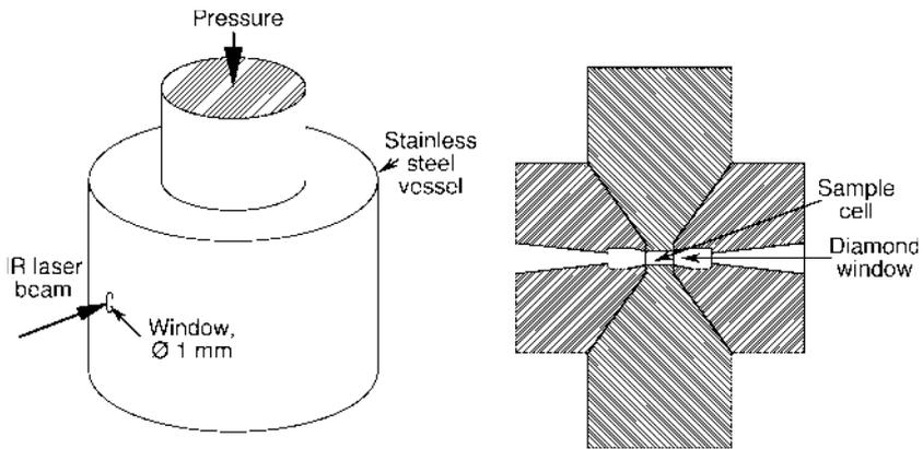
**Fig. 5.16** Apparatus to monitor protein unfolding under high pressure with IR. Since the volume of unfolded protein is less than that of folded protein, high pressure favors transition to the unfolded state
