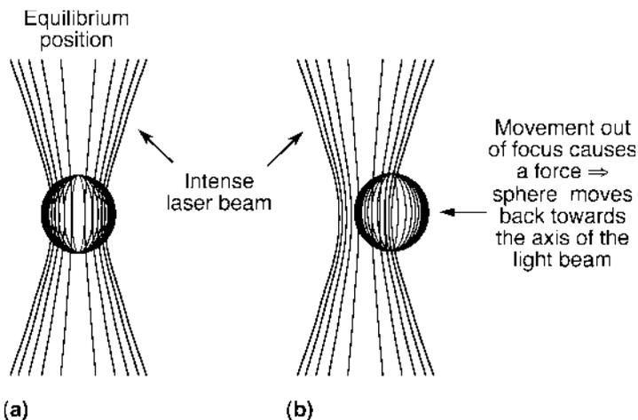
**Fig. 8.6** Optical tweezers for the measurement of the effect of template tension on T7 polymerase activity (Fig. 8.7; Smith et al., 1996; Wuite et al., 2000). Regarding the method of optical tweezers see also the groundbreaking studies of single-molecule mechanics by Florin et al. (Florin et al., 1997; Jeney et al., 2001; Pralle and Florin, 2002) and Smith et al. (Bustamante et al., 2000; Liphardt et al., 2001; Smith et al., 2001)
