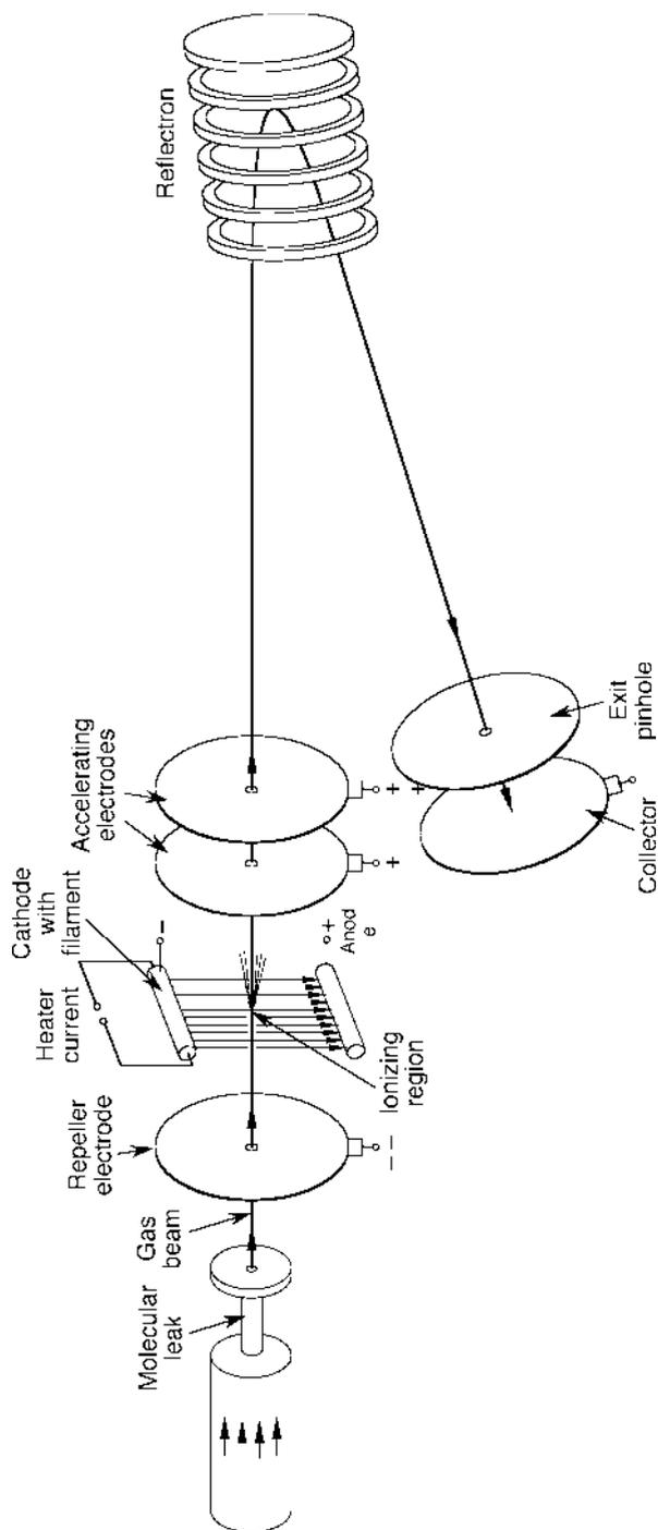
**Fig. 3.9** A high-resolution reflectron time-of-flight mass spectrometer. For further details see, e.g., IonSpec Corp., Irvine, CA; JEOL USA, Inc., Peabody, MA; Micromass and Waters Corporation, Milford, MA; Thermo Finnigan, San Jose, CA; Varian Instruments, Walnut Creek, CA
