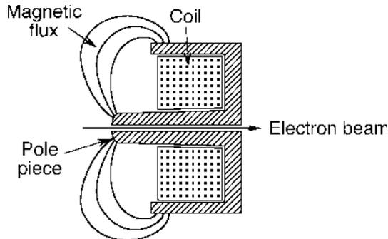
**Fig. 6.8** Ernst Ruska's pohlschuh lens: the circular electromagnet is capable of projecting a precisely circular magnetic field in the region of the electron beam
