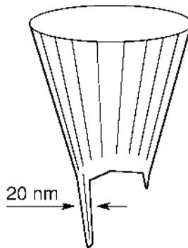
**Fig. 7.7** Tungsten tip, made by sharpening a tungsten wire by dragging it over a plate coated with alumina. This self-made tip may also be used for STMs (see Sect. 7.2)
