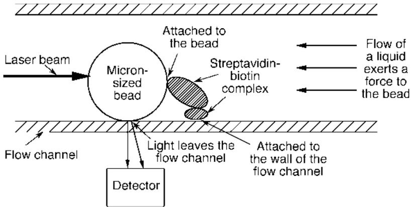
**Fig. 8.10** Force measurement on single molecular contacts through evanescent wave microscopy (Zocchi, 2001). The motion of the bead attached to the wall of the flow channel through a single streptavidin-biotin complex is tracked by detecting the evanescent wave as a force is exerted through a flow. This technique allows the direct measurement of the bond rupture force of the molecular complex
