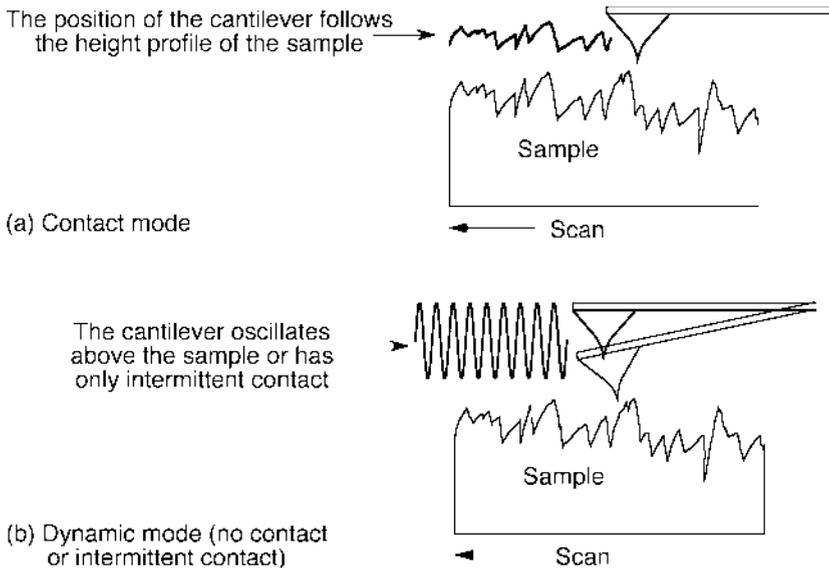
**Fig. 7.13** (a) Contact mode: the cantilever follows the height profile of the sample. (b) Dynamic mode: the cantilever has only intermittent contact or oscillates above the sample. In the latter mode, oscillations are excited by a piezo crystal and the forces between tip and sample are very small. This mode permits truly atomic resolution (Giessibl, 2000)
