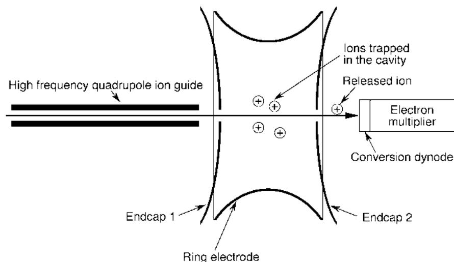
**Fig. 3.5** Ion trap mass analyzer. With the help of different radio frequency signals applied to the ring electrode and the endcaps, all ions are trapped in the cavity and then sequentially ejected according to their  $m/z$
