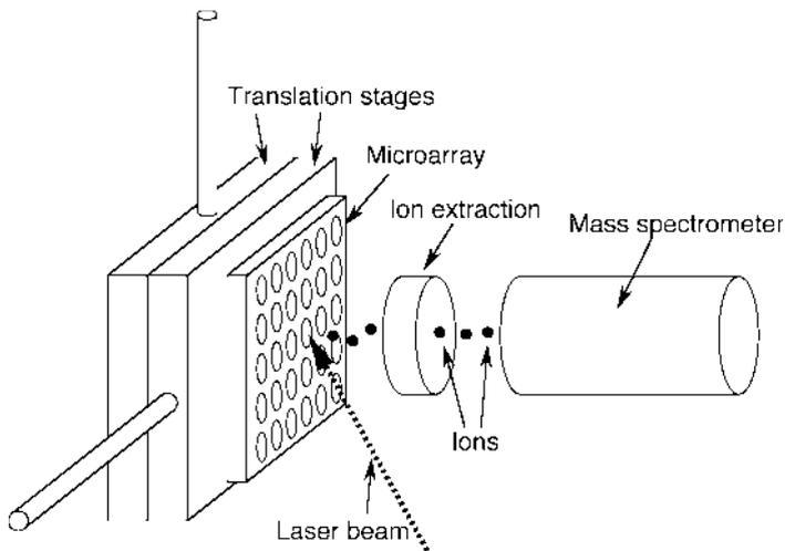
**Fig. 9.11** Mass-spectrometric array scanner for automatic mass-spectrometric measurement of protein and DNA microarrays. Step motor controlled translation stages rapidly move the microarray into position. A mass spectrum for each of the spots is automatically taken and analyzed. The scanner can be used, e.g., in the methods outlined in Figs. 9.5 and 9.6
