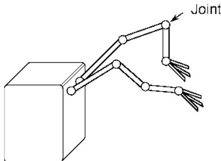
**Fig. 12.10** The calculation of movements of sophisticated robots can be connected with an exponential growth of possibilities with the degree of freedom of the system and accordingly such movements may be difficult to optimize
