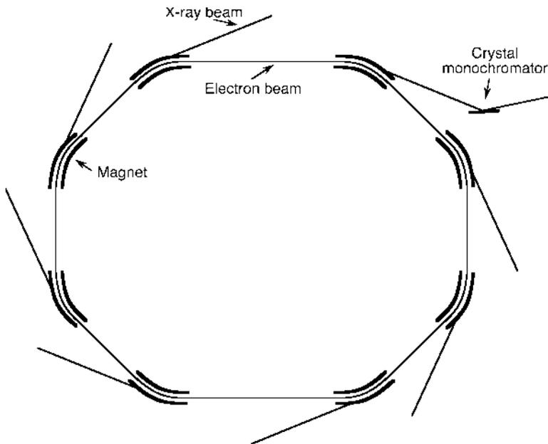
**Fig. 4.23** Design of a synchrotron. Ions or electrons are accelerated to a speed close to the speed of light and forced on a curved trajectory. A broad spectrum of radiation is produced along the curved sections of the beam. For protein crystallography, a certain wavelength, e.g., 1 Å, is selected by a monochromator
