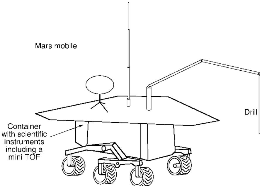
**Fig. 3.32** NASA plans to send rovers outfitted with MS to Mars. This sketch illustrates a mobile with mini-TOF searching for extraterrestrial life. Already now mass-spectrometry is utilized to search for extraterrestrial bacteria in meteors
