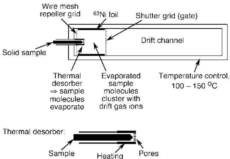
**Fig. 10.20** Modified IMS for the detection of chemicals contained in solid samples and for the identification of different solid materials, e.g., wood (Lawrence et al., 1991; Matz and Schröder, 1997; Schröder et al., 1998)
