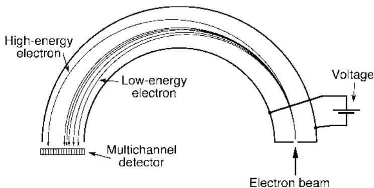
**Fig. 6.14** Determination of electron energies. The voltage applied between the two hemispherical electrodes disperses the electrons with respect to their velocity. In order to record a full spectrum for a large range of electron energies, the applied voltage is swept
