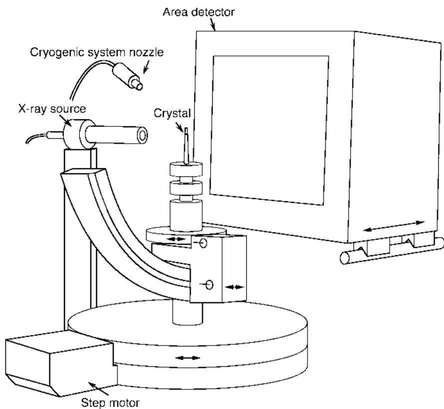
**Fig. 4.19** Setup for acquiring the diffraction pattern with an area detector (see, e.g., area detectors from Rigaku, The Woodlands, TX). The crystal is cooled with nitrogen from the cryogenic system nozzle. Cooling the crystal reduces radiation damage, but somewhat changes the intermolecular distances. Diffraction of the X-rays from the X-ray source by the crystal are recorded with the area detector with typically  $2048 \times 2048$  or  $4096 \times 4096$  pixels (see next figure)
