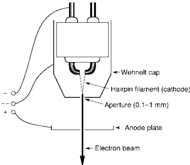
**Fig. 6.4** Thermionic electron gun (e.g., Structure Probe, Inc., West Chester, PA)
