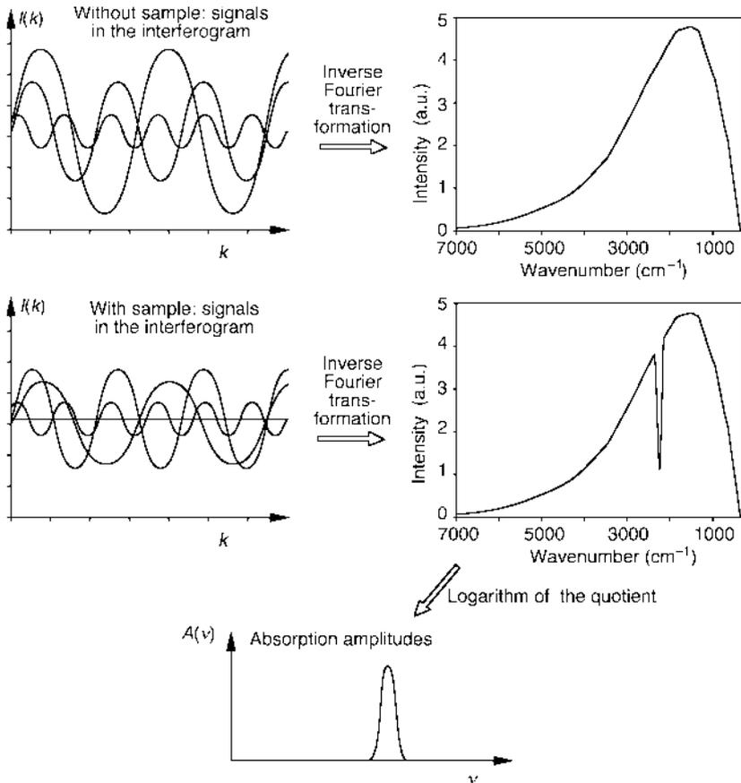
**Fig. 5.6** Principle of operation of a FTIR spectrometer. IR intensities at the detector are recorded both for the sample cell filled with solvent and for the sample cell filled with sample. Inverse Fourier transform of the two interferograms yields the IR intensities. The IR absorption spectrum is calculated using the logarithm of the intensity quotient
