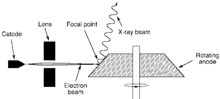
**Fig. 4.22** Rotating anode generator. An electron beam is focussed onto the rotating anode. It knocks out electrons from the inner electron shells of the anode metal. Reoccupation of the vacant shells by electrons from higher level shells involves the emission of X-ray radiation. The interaction of the electron beam with the anode metal generates also a large amount of heat which is quickly dissipated by rotating the anode below the spot of incidence of electrons
