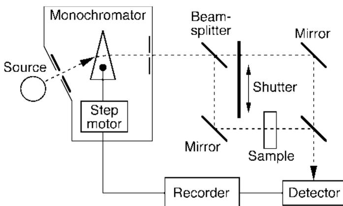
**Fig. 5.2** Example of a scanning infrared (IR) spectrometer. The monochromator separates the radiation of the IR source into its different wavelengths and selects one wavelength at a time. A beam splitter separates the monochromatic beam into sample beam and reference beam. The absorption coefficient, according to the chemical and structural properties of the sample molecules, is calculated using the detected intensity quotient between both beams, the pathlength, and the sample concentration
