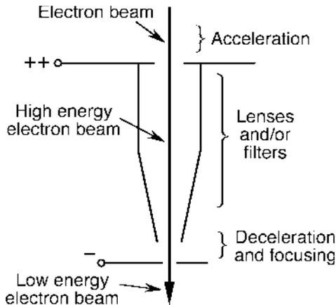
**Fig. 6.12** Beam booster (LEO Elektronenmikroskopie GmbH, Oberkochen, Germany). The electrons are accelerated to a high energy, passed through condenser lenses and filters, and then decelerated prior to interacting with the sample. This technique largely protects the electron beam against stray magnetic fields in the column of the microscope
