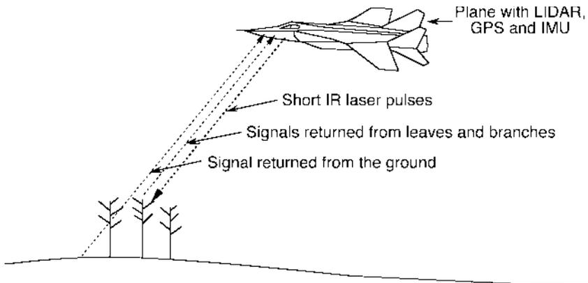
**Fig. 5.9** Remote survey of forest structure and terrain with IR LIDAR technology. The plane is equipped with a GPS and an inertial measurement unit (IMU). The latter contains several gyroscopes and an accelerometer and can determine the position and angle of tilt with some accuracy during periods of failure of the GPS
