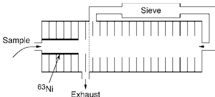
**Fig. 10.24** Improved purgeability of the reaction area (see, e.g., Snyder et al., 1993) and improved homogeneity of the electric field the ions experiencing in the drift channel: the sample outlet is located close to the shutter grid, and the diameter of the reaction area is smaller than that of the drift channel
