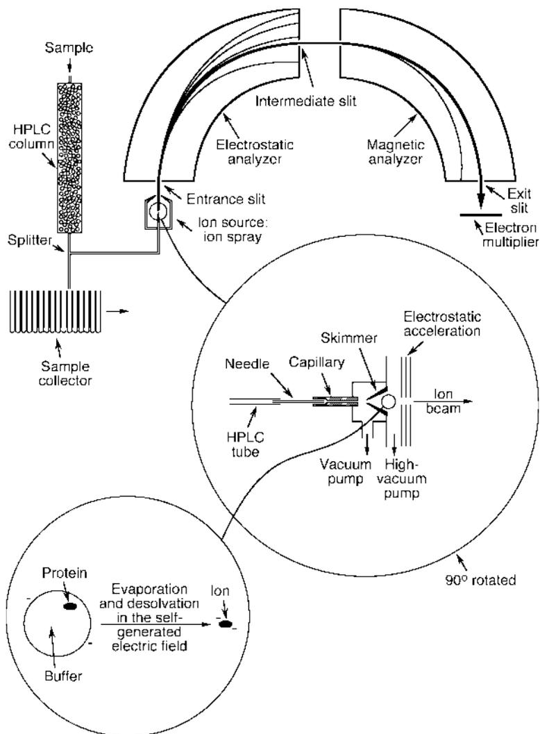
**Fig. 3.15** Double sector MS in combination with HPLC
