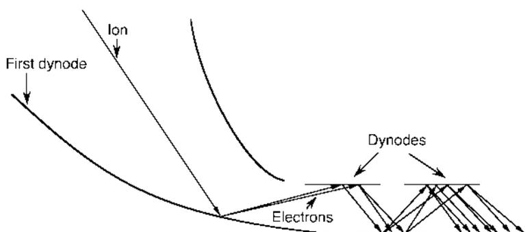
**Fig. 3.13** Electron multiplier for a MS. The first dynode converts the ion current into an electron current. Further dynodes amplify the electrons by a total factor of typically  $10^3$ – $10^8$ , largely dependent on the electron accelerating voltage between the dynodes, the number of dynodes, and the dynode composition. The last dynode is connected with an ammeter (not shown)
