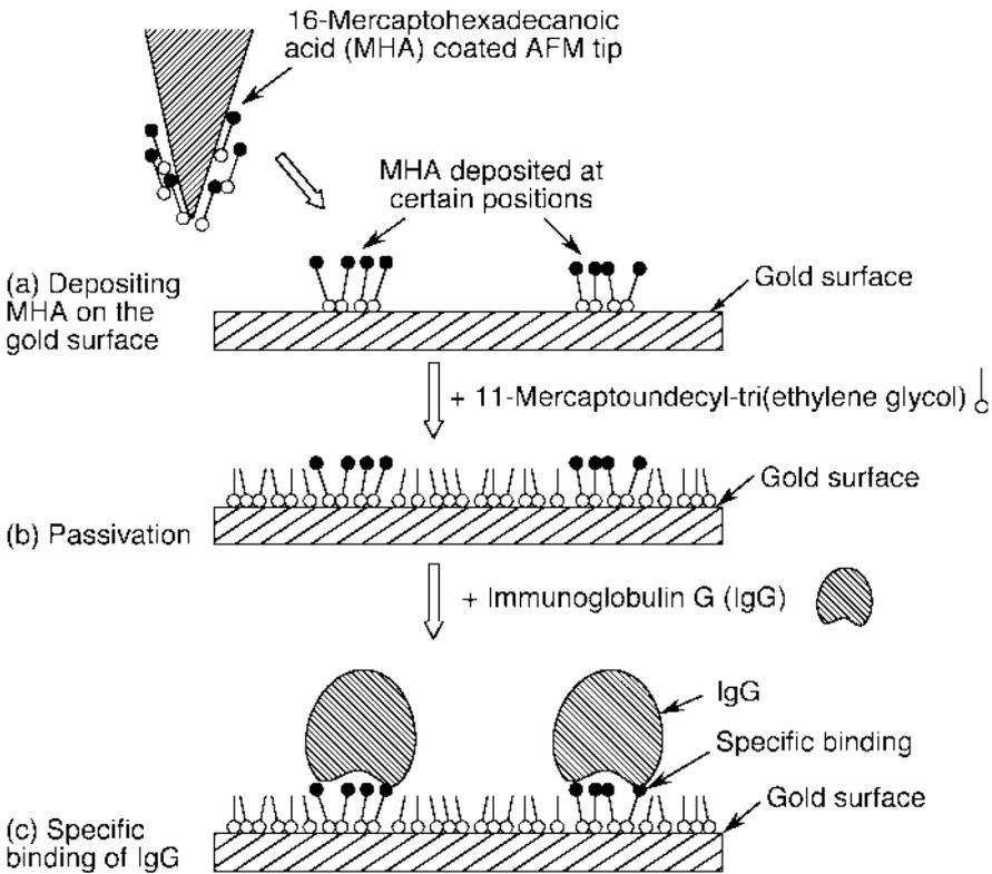
**Fig. 8.12** Manufacture of protein nanoarrays for the investigation of molecular interaction and other recognition processes (Lee et al., 2002b; see also Hodneland et al., 2002)
