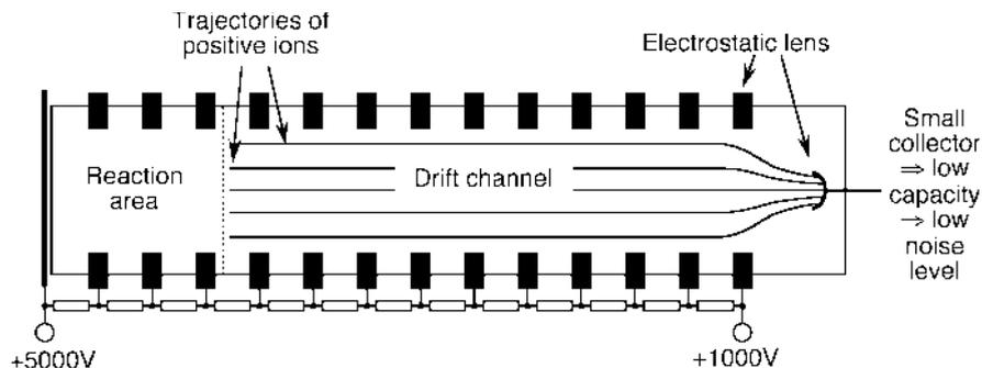
**Fig. 10.21** Noise reduction with a smaller collector grid: The collector and the guard ring in front of the collector act together as an electrostatic lens. The smaller collector causes less noise and, thus, a higher sensitivity
