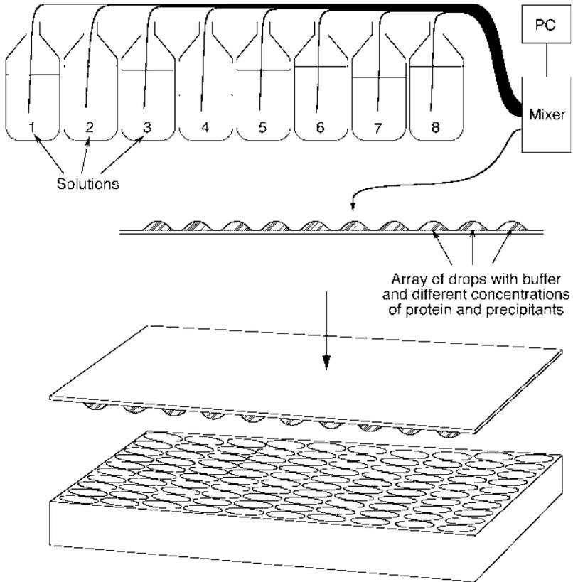
**Fig. 4.16** Crystallization robot for hanging drop crystallization. The computer-controlled mixer draws different solutions from reservoir bottles, mixes them with various ratios, and places the mixtures on a glass plate
