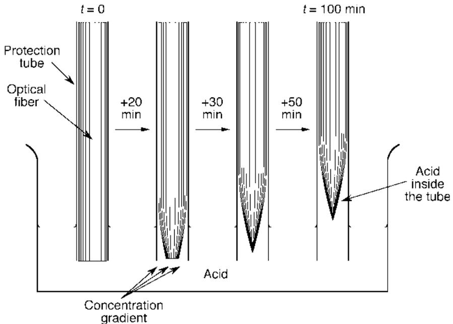
**Fig. 7.28** Tube-etching of a quartz glass fiber with hydrofluoric acid (Turner, 1983; Stöckle et al., 1999a, 1999b): the tip forms due to concentration gradients of acid and dissolved fiber. The tube serves also for suppression of convection of the acid. These tube-etched tips are inexpensive and have large cone angles permitting high light throughputs
