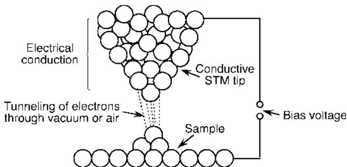
**Fig. 7.20** When the distance between conductive tip and conductive sample is lowered to a few Å, electrons can traverse the gap with some transmission probability. The STM measures not purely distance like the AFM, but the local density of electronic states
