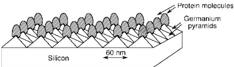
**Fig. 8.14** Protein nanoarray manufactured by self-assembly on nanometer-sized germanium pyramids (Riedel et al., 2001). Dynamic contact angle measurements with water droplets revealed that the germanium substrate is highly hydrophilic, and thus should be suitable for adsorption of hydrophilic proteins. Some protein inactivation was observed, however
