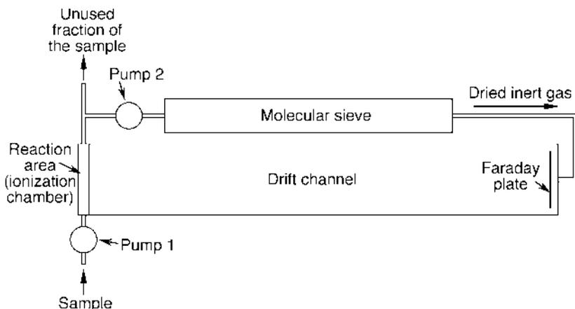
**Fig. 10.7** Drying the inert gas with a molecular sieve (Carnahan and Tarassov, 1998; Taylor and Turner, 1999). Suitable dimensions for a length of the drift channel of 5–20 cm, a diameter of the drift channel of 2–3 cm, and a height of the ionization chamber of 0.5–1 cm are: flow rate of pump 1: 5–50 ml min<sup>-1</sup>; flow rate of pump 2: 50–500 ml min<sup>-1</sup>
