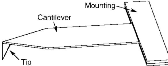
**Fig. 7.10** Sharp cantilever geometry for very rough samples (e.g., Olympus Optical Co., Tokyo)
