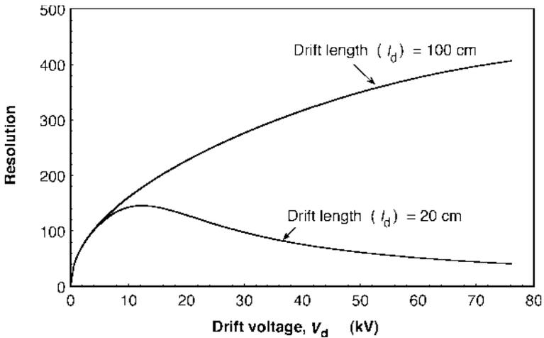
**Fig. 10.8** Theoretical resolution of an IMS at different drift lengths. At short drift lengths, increasing the drift voltage above an optimum does not further improve the resolution. The parameters in this example are: temperature, 130 °C; ion mobility,  $10^{-5} \text{ m}^2 \text{ V}^{-1} \text{ s}^{-1}$ ; initial ion pulse width, 1 ms; shutter pulse voltage, 1000 V; length of the reaction area, 3 mm; distance between aperture grid and Faraday plate, 1 mm; voltage at the aperture grid, 500 V
