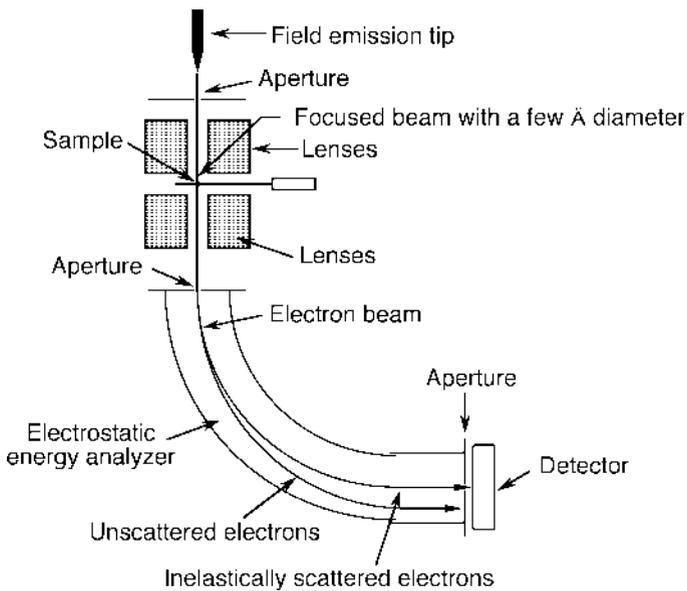
**Fig. 6.20** Example of a scanning transmission electron microscope with an energy filter: inelastically scattered electrons, i.e., those which have changed both energy and direction upon interaction with the specimen, are collected yielding the inelastic dark field image. Electrons with different energies are separable by their trajectories with different curvatures in the electric field applied perpendicular to the flight direction
