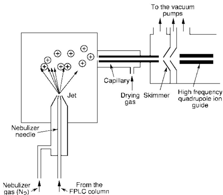
**Fig. 3.18** FPLC/MS connector. In several stages the solvent is removed from the analyte solution by application of dry nitrogen and vacuum. The quadrupole ion guide leads the ions to the mass analyzer of the mass spectrometer
