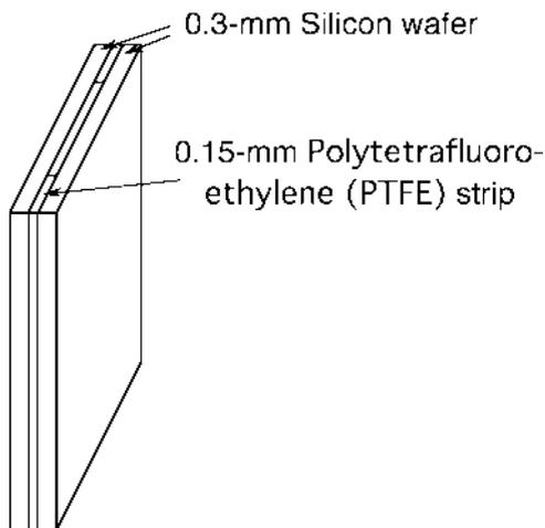
**Fig. 5.7** Sample cell for FTIR experiments. The transparent walls of the cell are made from silicon wafers supplied by a manufacturer of electronic chips
