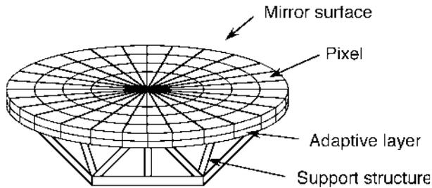
**Fig. 12.8** Adaptive systems are used in optics, e.g., to compensate for bending of the support structures of large mirrors due to its own weight and thermal fluctuations and for the distortion of the image by density fluctuations of the atmosphere
