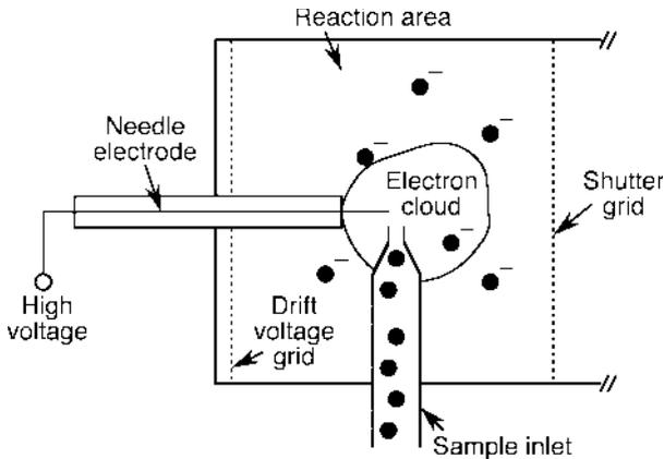
**Fig. 10.16** Gas inlet for electrical-discharge (corona discharge) ionization
