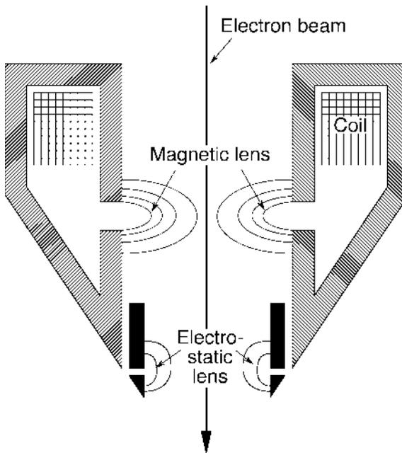
**Fig. 6.10** Compound lens made from magnetic and electrostatic lenses: the magnetic field forces the electrons on spiral-shaped trajectories; the electric field further decreases the diameter of the electron beam. Additional coils may serve for the correction of spherical aberration (not shown)
