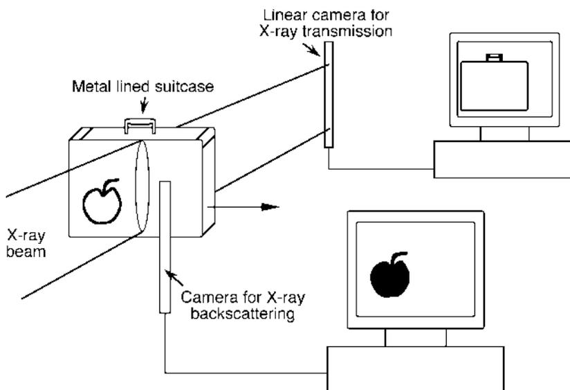
**Fig. 4.40** Detection of biological and other organic material behind a metal layer with X-ray backscattering: since the absorption of biological material is much smaller than that of metal, the biological material is difficult to detect in single-wavelength X-ray absorption measurements. X-ray backscattering provides much better contrast in this application. However, the quantum efficiency of X-ray scattering is low and thus relatively large exposures and sensitive cameras must be used
