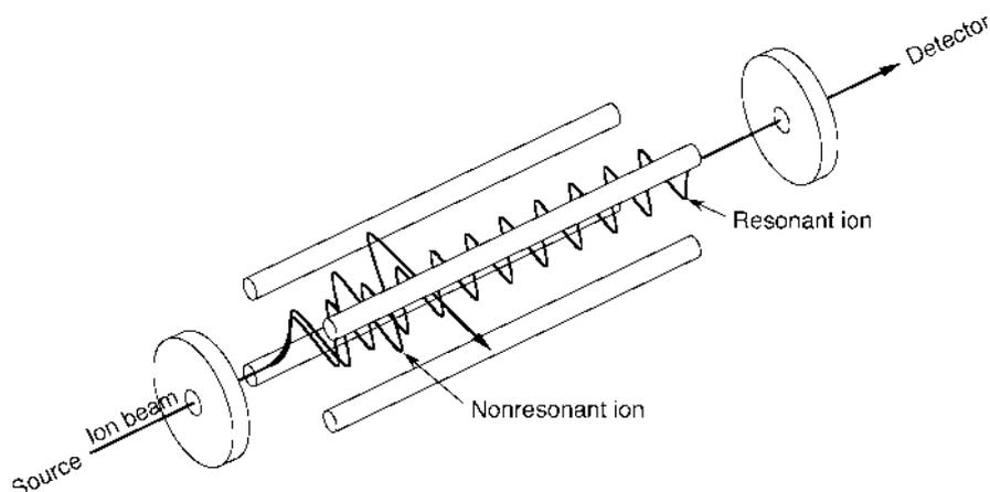
**Fig. 3.4** Quadrupole mass spectrometer. The ion beam is accelerated to a high velocity by an electric field and passed through the quadrupole mass analyzer comprising four metal rods. DC and AC potentials are applied to the quadrupole rods in such a way that only ions with one mass-to-charge ratio ( $m/z$ ) can pass through the analyzer at a time. To scan different  $m/z$ , DC and AC potentials are varied
