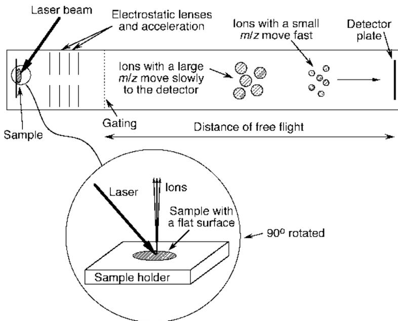
**Fig. 3.6** Linear time-of-flight mass spectrometer (TOF) with matrix-assisted laser desorption ionization (MALDI). The linear configuration of TOFs represents the simplest implementation of the time-of-flight technique. The typical mass range lies between 0 and 100 kDa, and the typical mass resolution  $m/\Delta m$  is 300–2000
