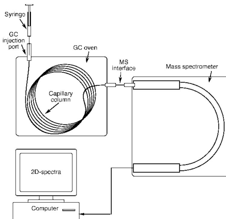
**Fig. 3.16** GC/MS. The combination of mass spectrometry with gas chromatography can greatly enhance the resolution of complex samples
