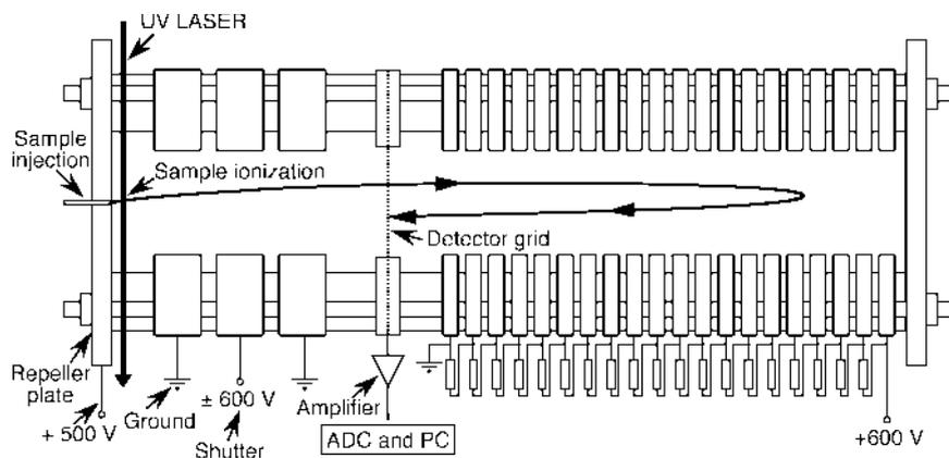
**Fig. 3.7** A simple reflectron time-of-flight mass spectrometer (e.g., Bryden, 1995). The reflector enhances mass-spectrometric resolution: it increases the time of flight and can focus ions. Here a voltage pulse at the shutter electrode causes a uniform starting time of the ions
