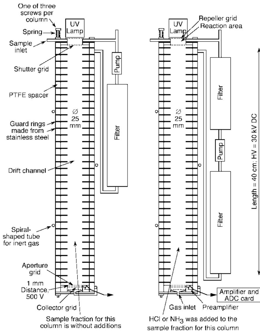
**Fig. 10.18** A high-resolution two-channel ion mobility spectrometer. Here the sample is simultaneously analyzed in two different ways reducing false identifications of agents. In one of the columns, the sample is chemically and/or physically modified by a chemical addition
