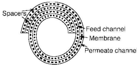
**Fig. 2.17** Side view of a spiral cartridge concentrator (e.g., Millipore Corporation, Bedford, MA). Pressure is applied by centrifuging the concentrator. Similarly to the pervious ultrafiltration device (Fig. 2.16), small molecules pass the membrane and large molecules are retained
