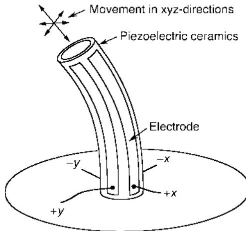
**Fig. 7.5** Principle of operation of the xyz-piezoelectric scanner, a ceramic positioning device which changes its size in response to a change in applied voltage. A voltage change at the  $x$ - or  $y$ - electrodes causes bending in the horizontal plane; contraction and expansion are generated by simultaneous application of  $x$ - and  $y$ -voltage
