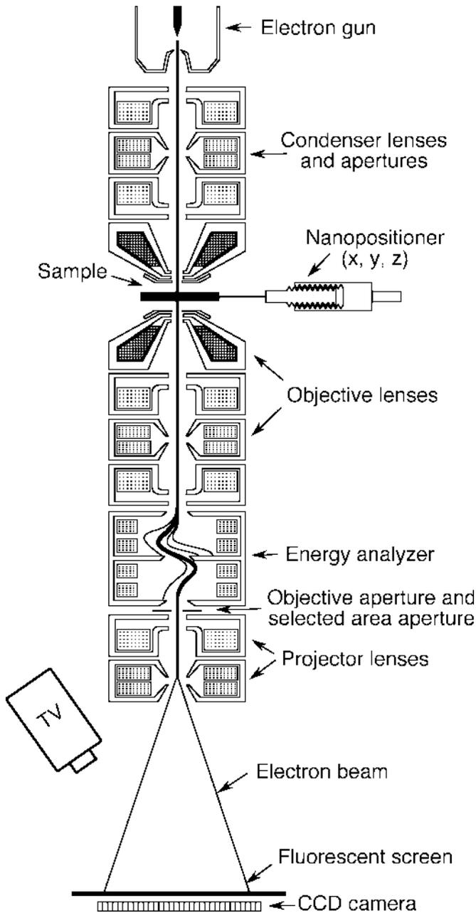
**Fig. 6.2** A more complicated design of a transmission electron microscope with an analyzer which can remove inelastically scattered electrons (see, e.g., LEO Elektronenmikroskopie GmbH, Oberkochen, Germany)
