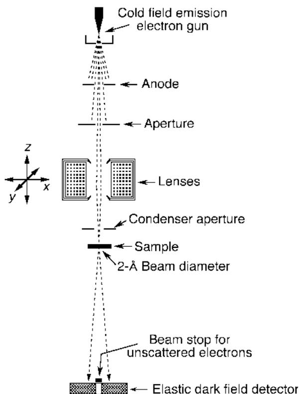
**Fig. 6.19** Scheme of a scanning transmission electron microscope: The objective lens focuses the electron beam onto a small sample section. Scattered electrons are detected with the elastic dark field detector. The STEM image is generated by moving the focussed beam over the specimen
