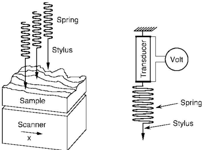
**Fig. 7.2** Stylus profilometer for comparison with the AFM. A set of styli probes the sample which is drawn below the set of styli. The small motions of the styli are transformed into an electrical signal by linear, variable transducers. Step heights of down to a few 10 nm are resolvable
