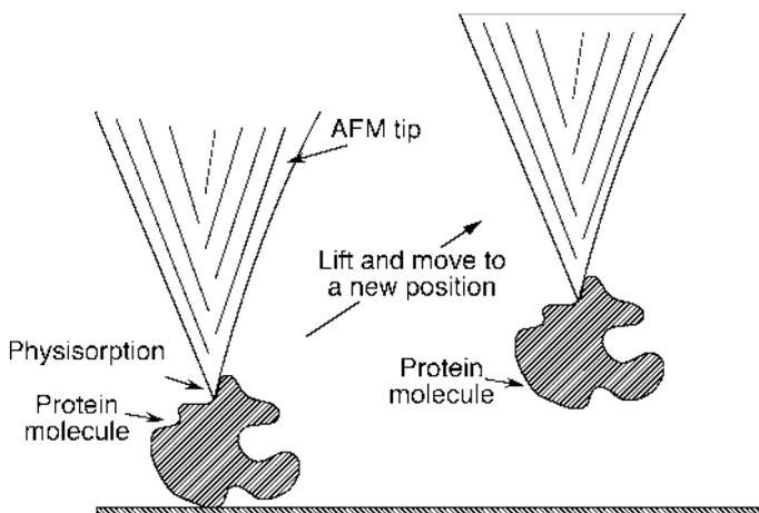
**Fig. 7.18** Manipulation of a protein molecule with an AFM: The tip is lowered till it touches the macromolecule. Due to the attractive action of the van-der-Waals interaction, the macromolecule sticks to the tip and can be lifted and moved to a different place
