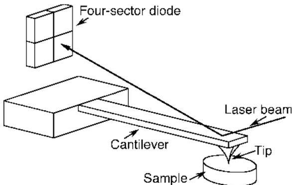
**Fig. 7.34** Example of a friction force microscope: the detector has sectors in both vertical and horizontal direction so that the torsion of the cantilever can be estimated and a frictional (lateral) force be calculated (see, e.g., Howald et al., 1995)
