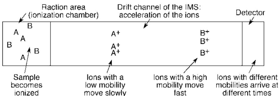
**Fig. 10.1** Principle of operation of ion mobility spectrometers: Molecular ions are generated and accumulated in the reaction area. A gating pulse transfers the molecular ions to the drift channel where said ions are accelerated by an electric field. Ions with different mobilities in the gaseous medium of the drift channel arrive at different times at the detector
