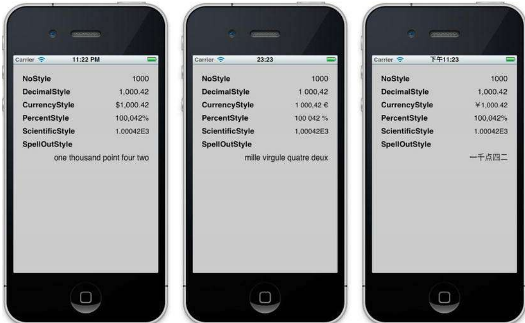
Figure 12-3. Our example app running in the United States locale (left), French ► France locale (center), and Chinese ► China (right)
