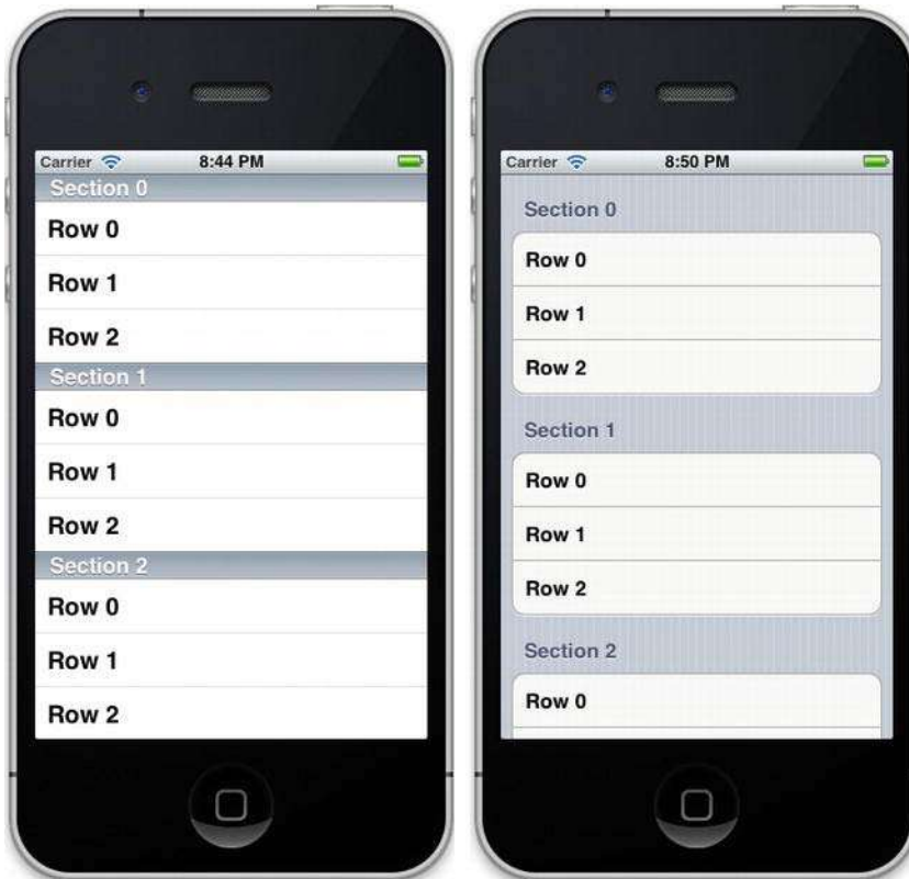
Figure 3-4. A prototypical UITableView . On the left is a table view with the “plain” style, and on the right is the “grouped” style.
