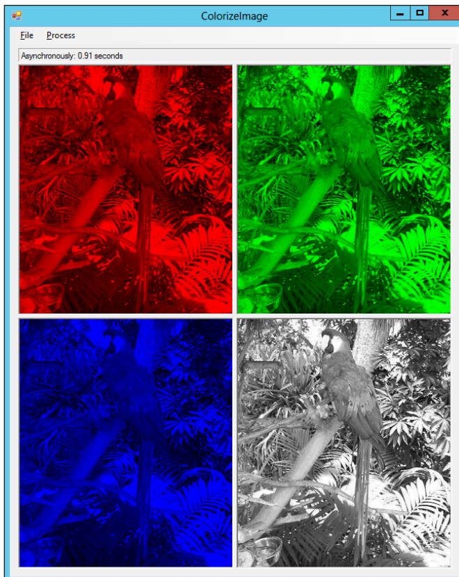
FIGURE 6-3: The ColorizeBitmap example program creates red, green, blue, and gray versions of an image synchronously and asynchronously.
