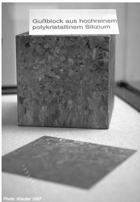
**Fig. 6.2.** Ingot of multi-crystalline silicon (formerly known under the name of “poly-crystalline silicon”) with square cross-section.
