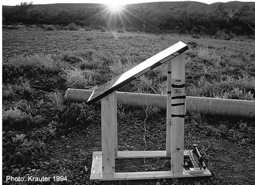
**Fig. 7.24.** Experimental set-up for the validation of the thermal and optimal modeling at a research station of the University of New South Wales at sunrise (Foulders Gap, Australia, 31° S, 140° E). Clearly visible are the high optical losses caused by the reflection of the flat incidence of the direct component of irradiance.
