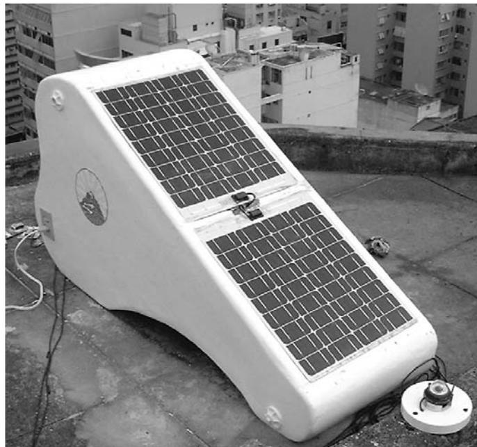
**Fig. 10.26.** The Integrated SHS (I-SHS) prototype during tests in Copacabana, Rio de Janeiro, Brazil. Modified design of “Escola de Belas Artes”, UFRJ, Rio de Janeiro.
