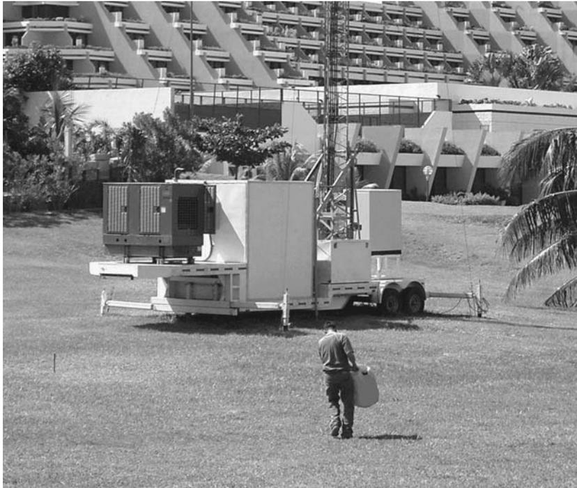
**Fig. 5.1.** Diesel powered generator for the supply of a 2 kW cellular phone repeating station with noise and exhaust gases in a hotel area in Cancun, Mexico. Operation personnel has to arrive every 12 hours to do a refill – why not PV?
