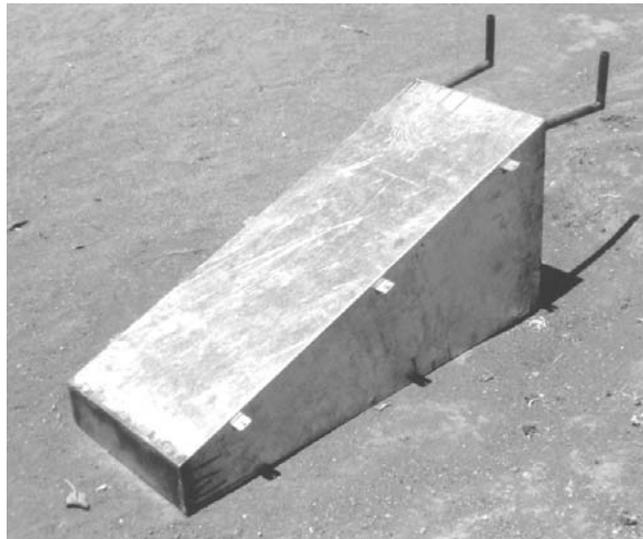
**Fig. 10.20.** Tank for reduction of cell temperature and serving as module mount/foundation, manufactured in Harare (Zimbabwe) by galvanized sheet steel (without internal convection aid).
